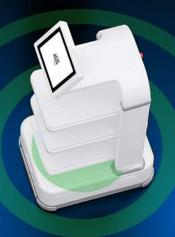
Our robot plans its work according to the current charge/power balance. If it calculates that it cannot finish its task in the area where it will perform autonomous navigation, it first goes to the charging unit and recharges, then continues its task.
